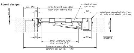
Fig. 2 – SD7.R embedded in concrete
