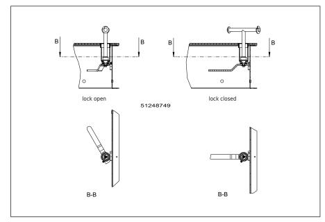
Fig. 12 – SD7 lock with opening possibility from below
