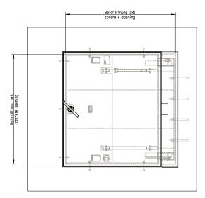
Fig. 5 - SD7 (15kN) for bolted fixing
