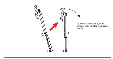
Fig. 11 – Unlocking the arrester of the gas pressure spring
