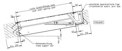
Fig. 3 – SD7 Inclined istallation
